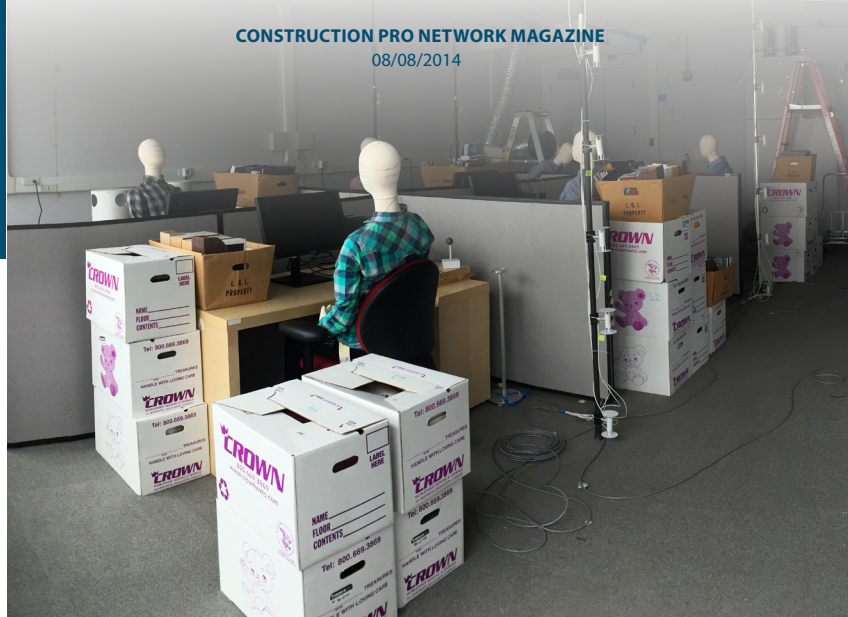
Experiment cell space showing an office configuration with added books representing heavy internal thermal mass.
